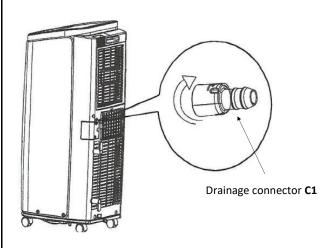
**STEP 3.** Securely attach Drainage Hose **C2** (14mm) into the drainage connector.
