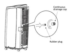
**STEP 2.** Fasten the Drainage Connector **C1** to the drainage port (turning clockwise).
